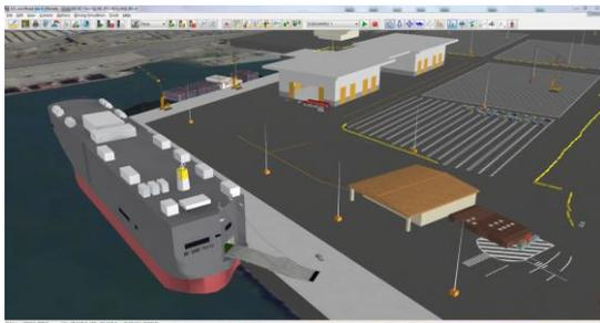
The PCC simulator consists of a drive simulator with a 3D virtual model of a PCC ship and the yard (or wharf) to which the vehicles are unloaded and parked. The 3D virtual model was developed in Forum8 software UC-win/Road; as well a special plugin was developed for the driver training and assessment function.
