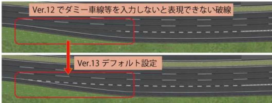
Fig. 5 A flexible designing of carriageway. A dash line rendering that required the dummy carriageway setting in the Ver. 12 can now be displayed by the default setting in the Ver.13.
