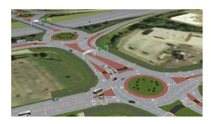
UC-win/Road was able to provide a practical solution whereby the public could drive through the planned roundabout in virtual reality. Using USB steering wheel with UC-win/Road, members of the public were able to drive on the proposed roundabouts first hand. In the photo-realistic and spatially-accurate environment of UC-win/Road, drivers could understand exactly what their journey to work would be like after these roundabouts were built.
