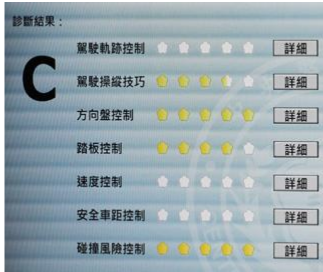
After driving, the comprehensive driving skill, car distance keeping, collision possibility and other details are scored.
