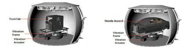
The engine was removed from the Honda Accord to be replaced with equipment such as the electronic control system and an acoustic PC. A PC power and a connection terminal for the Internet were also positioned inside the cabin. The original vehicle's steering wheel and accelerator / brake pedals were retained to help achieve the real driving sensation.
